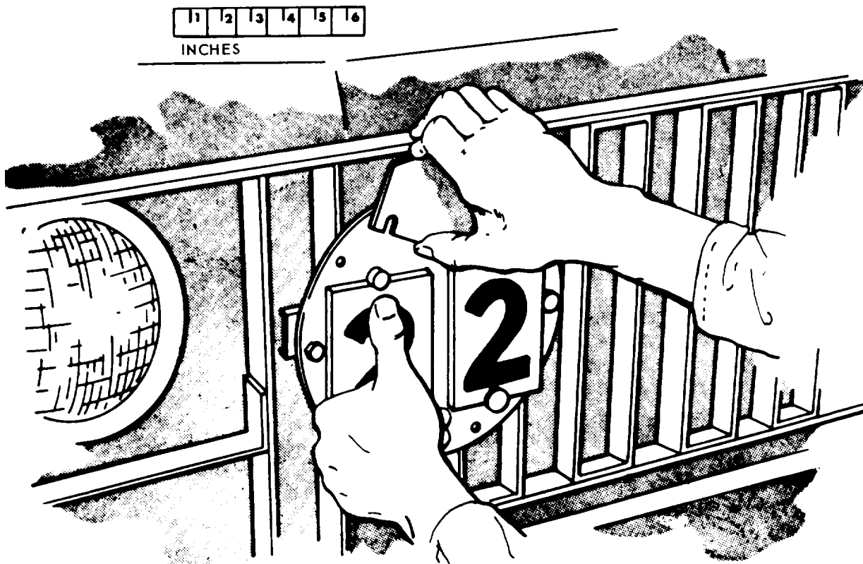
Figure 2-8. Unlocking the retaining plate.
